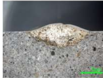
Cross section of coating III
